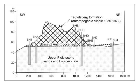
**Figure 2.** The Teufelsberg Formation (sensu Leinfelder and Scheffold, unpubl.) of war rubble including concrete, brick, clinker, rock, fly ash, slag and solid chemical waste, deposited between 1950 and 1972, forming the highest elevation of Berlin. Thin Holocene deposits may locally separate the Pleistocene and Anthropocene units.
