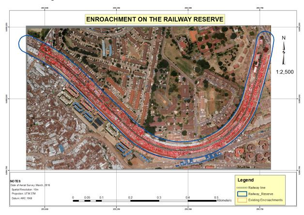
Figure 3: Structures encroaching on the Railway Reserve within Soweto East
