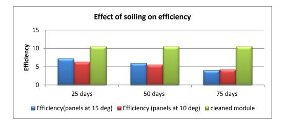
Figure 4.7: Effect of soiling on efficiency
