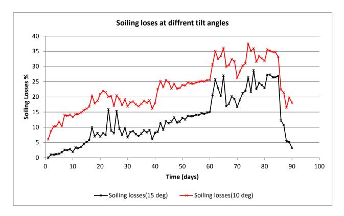
Figure 4.8: Soiling losses for the PV panels at different tilt angles
