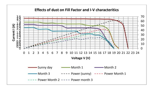
Figure 4.6: Effects of soiling on FF, Power and I-V over the study period
