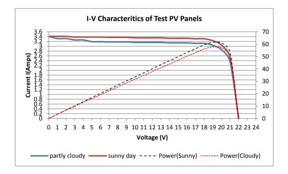
Figure 4.4: The I-V characteristics of the tests panels
