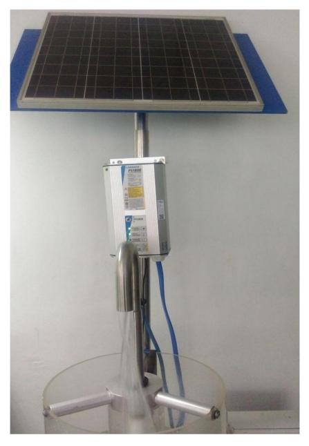
Solar water pumping system with flow meter and controller
