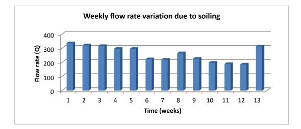
Figure 4.9: The weekly variation in Flow rate due to soiling
