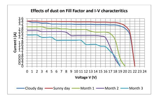
Figure 4.5: Effect of soiling on I-V characteristics and Fill Factor
