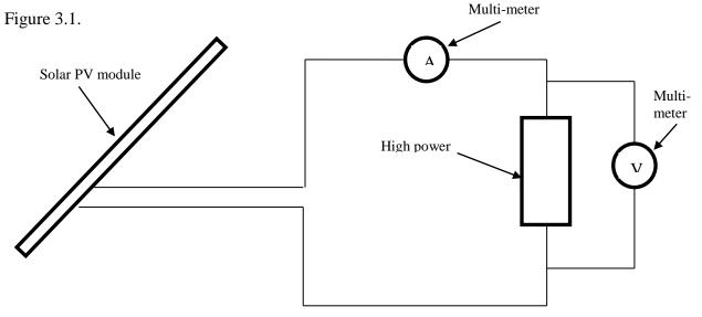
**Figure 3.1: Experiment test and calibration circuit**
