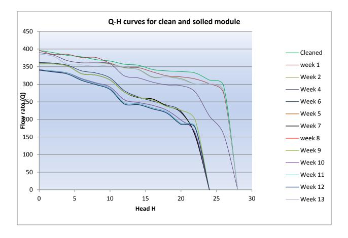
Figure 4.10: Variation in Q-H curves due to soiling
