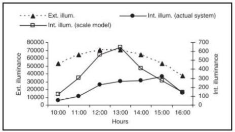
Figure 4.10: Test performance for a 560mm Diameter, 25M Length light pipe Source: Solartube, UK
