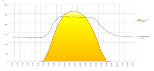
Figure 4.15 (b): Lighting load Profile vs. Projected Solar PV Generation
