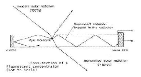
Fig 2.10: Cross-section of a fluorescent concentrator.
