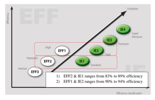
Figure 2.5: World standard motor efficiency classification
