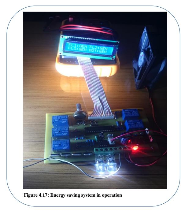
Figure 4.17 shows the display from the LCD that, Floor 1, 2, 3 and the motor are all powered by the Standby Generator. This is a situation whereby in case there is no power from mains and from solar as well Generator should take on the full load.
