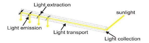
Figure 2.7: Light piping system diagram
