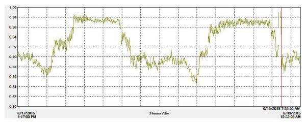
Figure 4.20: Logged power factor for Lift 1
