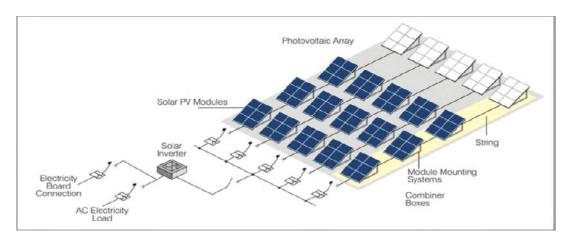
Fig 2.2: Typical Solar PV System Architecture
