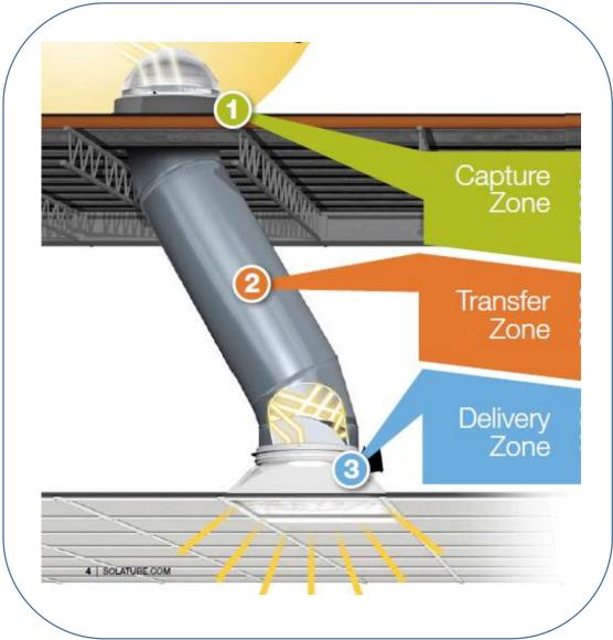
Fig 2.8: Typical Light-pipe system
