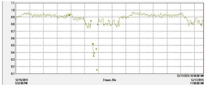
Figure 4.21: Logged Power Factor for Lift 2.
