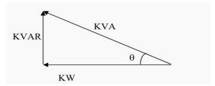
Figure 4.18 (b): Power Factor Vector diagram
