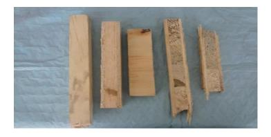
Figure 3.1.4: Blockboard sample
