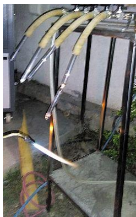
Figure 4.6: sealing of ingots in quartz tubes for annealing
