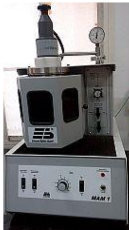
Figure 3.3: Photograph of the Arc melting furnace at IIT, Mandi Laboratory
