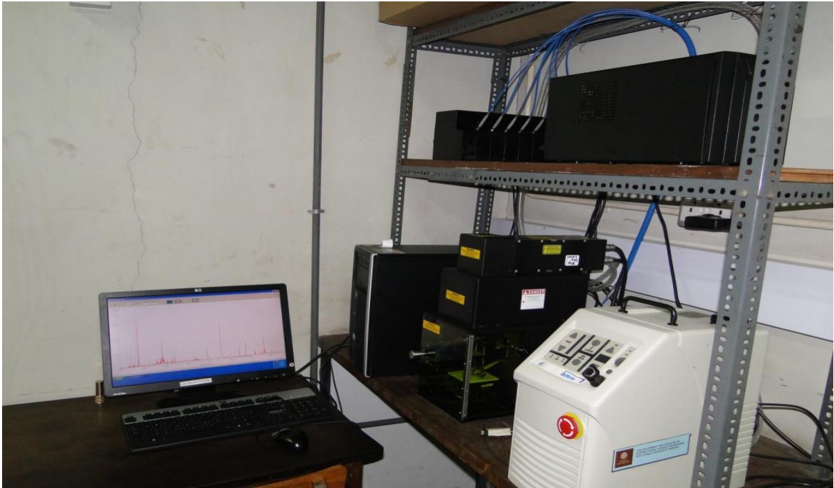
Figure 4.3: Photograph of the LIBS 2500 PLUS (Ocean Optics) used while carrying out the research.
