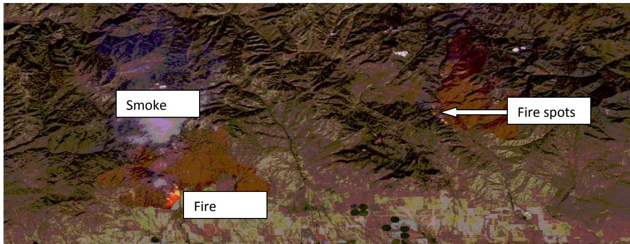
Figure 4.3. Resultant image when 2r - g - b is used on the MODIS image.
