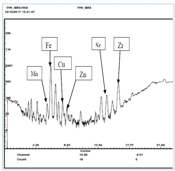
Figure 5.1: Spectra of PTXRF IAEA 09 reference soil sample
