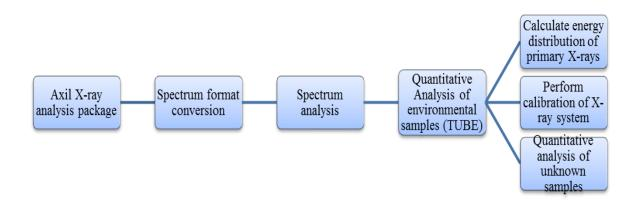
Figure 4.3: Block diagram showing the steps followed in Axil spectral analysis
