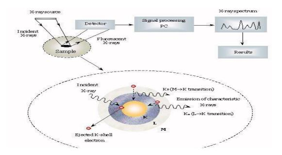
Figure 3.1: The principle of XRF and the typical XRF detection arrangement (Andrew, Keith, 2013).
