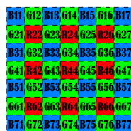
Fig. 1. A 7-by-7 window of the Bayer CFA Pattern (US Patent 3971605)
