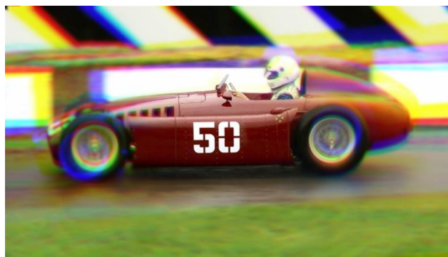
Figure E.2 Image illustrating chromatic aberration
