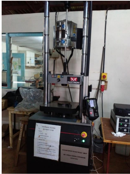
Figure 3.10. The Instron 300Dx universal testing machine (UTM) used for tensile testing.
