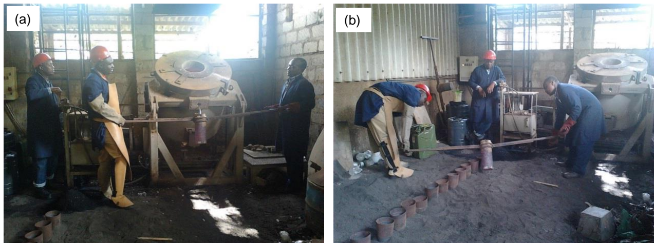
Figure 3.1. Pouring of the cast aluminium melt into (a) a preheated ladle and then (b) the ingot steel moulds.
