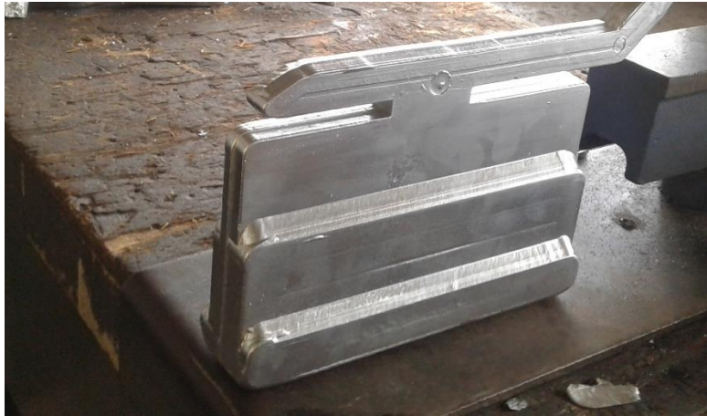
Figure 3.1. The bar casting obtained after the melt had solidified inside the permanent mould.
