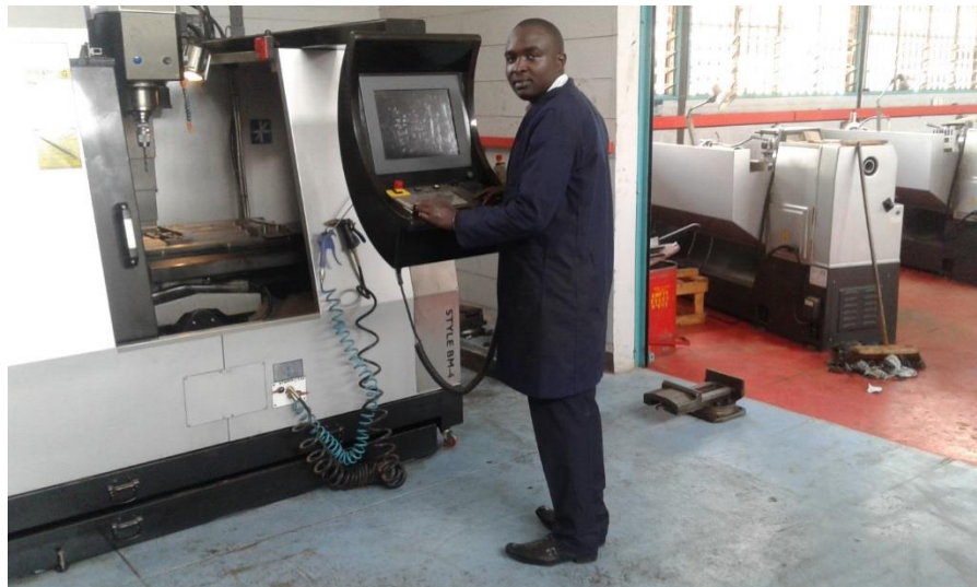
Figure 3.5. The computer numerically controlled (CNC) milling machine used to machine the permanent mould.
