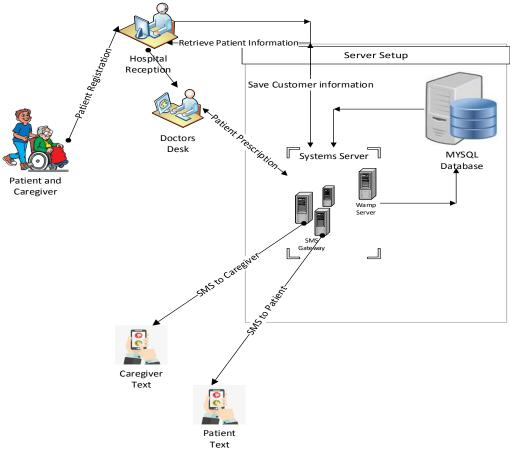
*Figure* **5.0**: *Prototype Architecture* (**Source**: This study)
