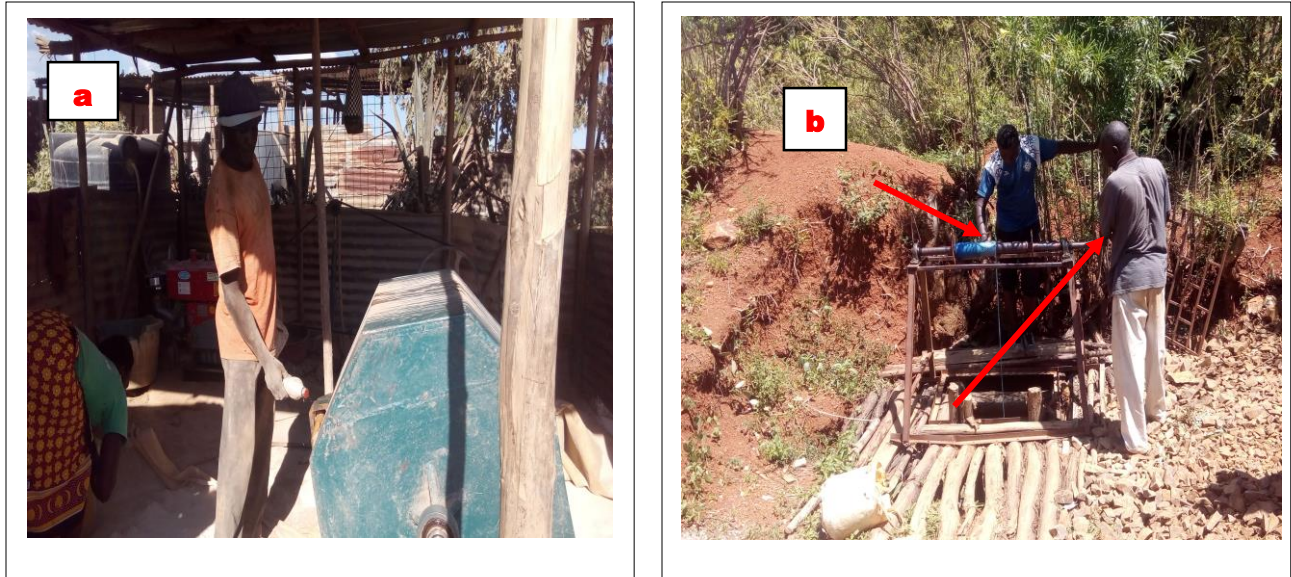
Plate 4.3: Equipment Use; (a) A miner repairing a crusher whilst it is operating and without relevant PPEs and (b): Miners operating a winch without appropriate PPEs
