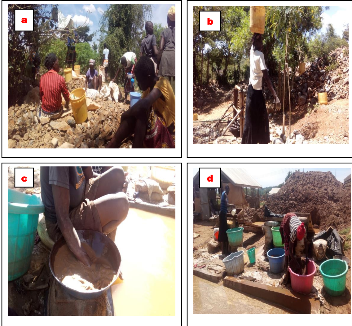
Plate 4.4: Female miners and the use of PPEs; (a) Female miners breaking rocks on site without appropriate PPEs, (b) A female miner carrying rocks on her head without appropriate PPE, (c) A female miner stirring slurry without protective gloves & (d) Female miners sluicing and panning soil without relevant PPEs.
