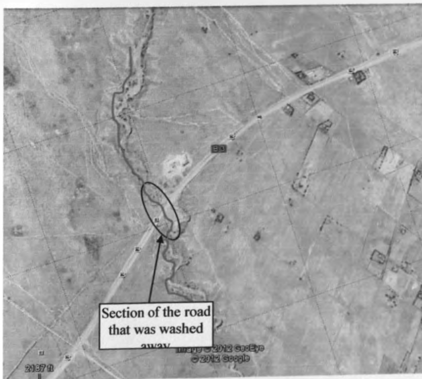
Figure 4.27: Section of the Maai Mahiu – Narok that was Washed away by Floods
