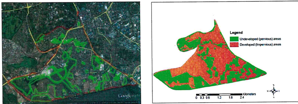
Map 2a and 2b: Digitizing pervious and impervious areas of the study area (Nairobi West and South C).
