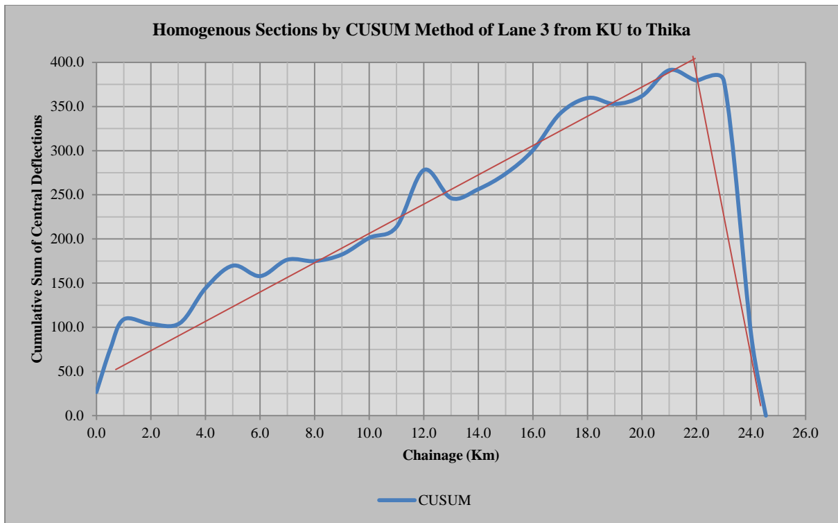
Figure 4.14: Homogenous Sections on Lane 3 from KU to Thika
