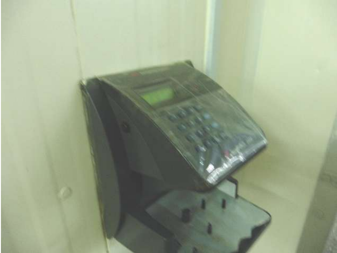
Plate 6.1: The biometric clock- in and out device ( Bonyeza ) for labor management (Photo taken by Author, 2017)
