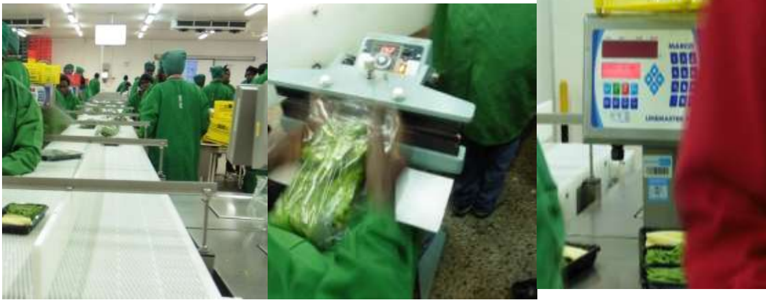
Plate 4.2: Pictures capturing grading, packaging, weighing and sealing of produce in the pack-house along the conveyor belt circuit. (Photos taken by author, 2017)
