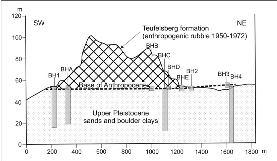
**Figure 2.** The Teufelsberg Formation (sensu Leinfelder and Scheffold, unpubl.) of war rubble including concrete, brick, clinker, rock, fly ash, slag and solid chemical waste, deposited between 1950 and 1972, forming the highest elevation of Berlin. Thin Holocene deposits may locally separate the Pleistocene and Anthropocene units.
