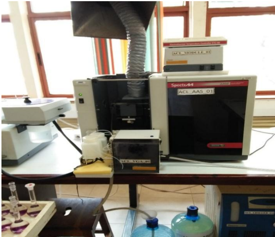
Figure 6: The Varian Model Spectr AA 220Z atomic absorption spectrometer fitted with Varian Model vapour generation accessory (VGA) 77 used for the analysis.
