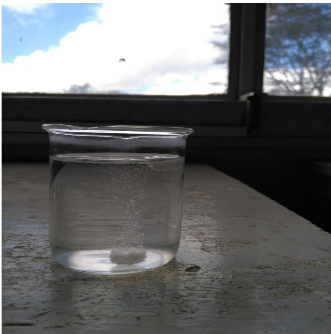
Figure 4.5: Continuous bubbling from a preliminary dosage unit containing 24% w/w polymer proportion
