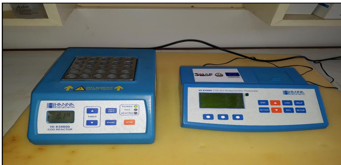
Figure 3.3: COD reactor and Multiparameter photometer
