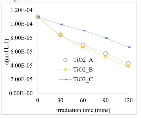
Fig 9: Degradation of 4-Chlorophenol using selected TiO<sub>2</sub> catalysts calcined at 550°C
