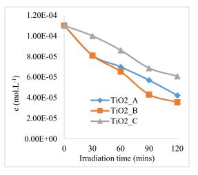
Fig 10: Degradation of 4-Chlorophenol using selected TiO<sub>2</sub> catalysts calcined at 600°C
