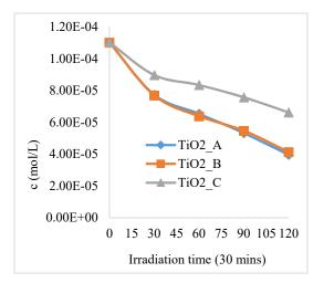
Fig 12: Degradation of 4-Chlorophenol by  $TiO_2$  catalysts annealed at  $700^{\circ}C$
