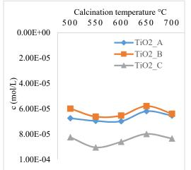
Fig 14: Changes in 4-chlorophenol concentration with selected  $TiO_2$  catalyst after 1 hr. of photocatalytic degradation
