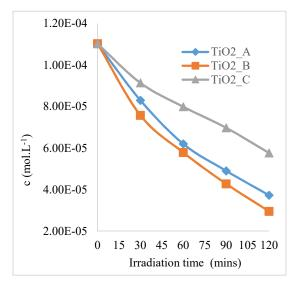
**Fig 11**: Degradation of 4-Chlorophenol using selected TiO<sub>2</sub> catalysts annealed at 650°C.
