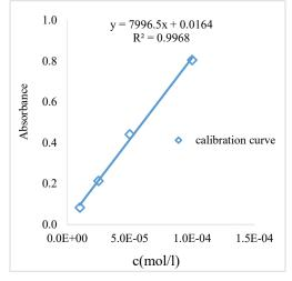
**Fig 7**: Calibration curve 4-chlorophenol
