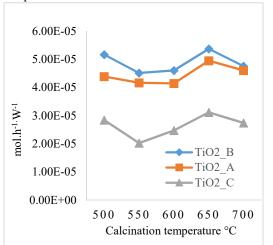
**Fig 13**: Effect of  $TiO_2$  catalyst calcination temperature on the rate of 4-Chlorophenol removal after 1 hour of photocatalytic treatment.
