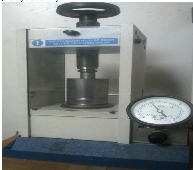
Figure 3.3: The hydraulic press complete with the die assembly
