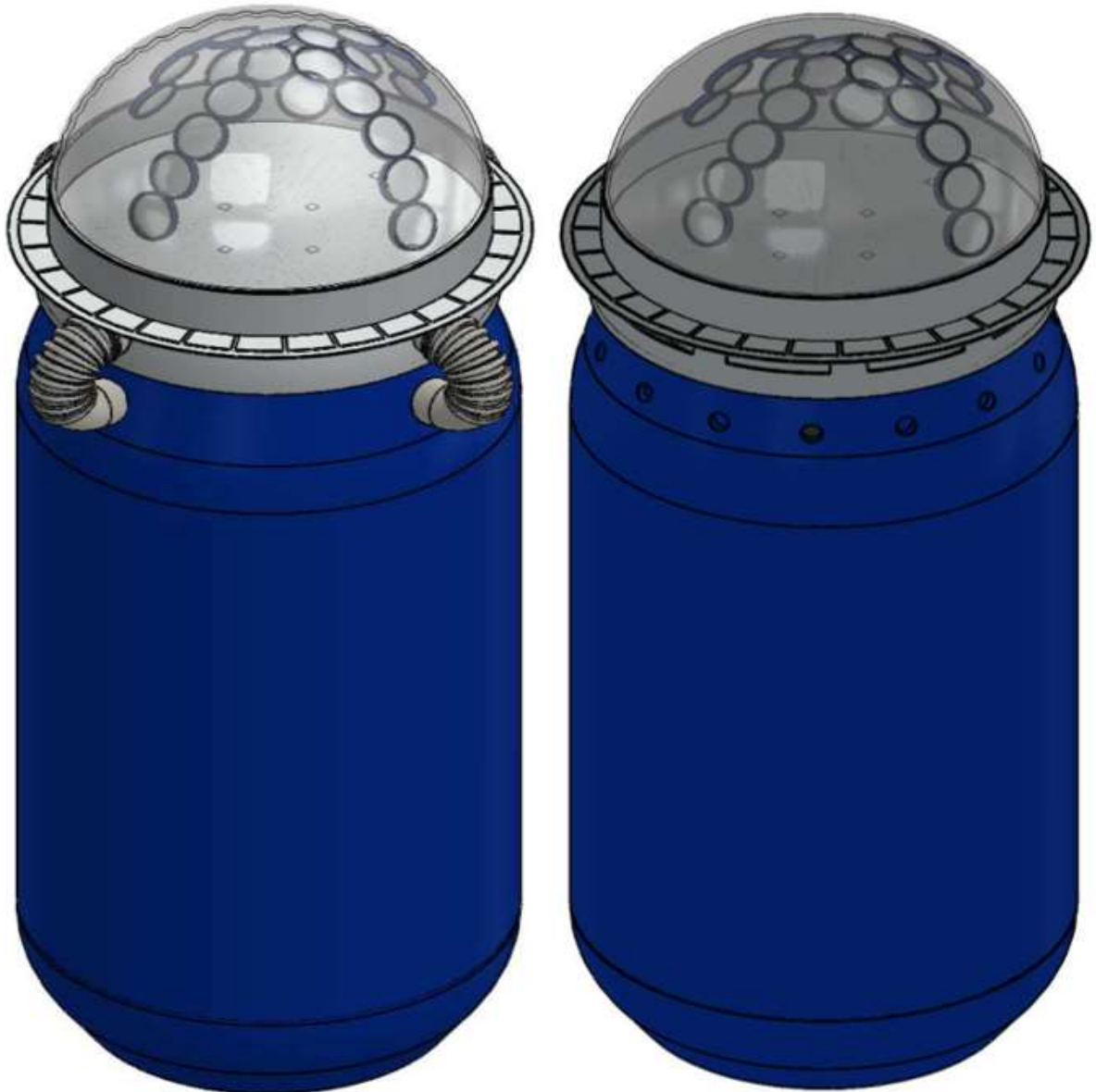
Plate 8-8: Desiccant exhaust recirculation dryer and Ambient inlet-outlet dryer (single pass)
