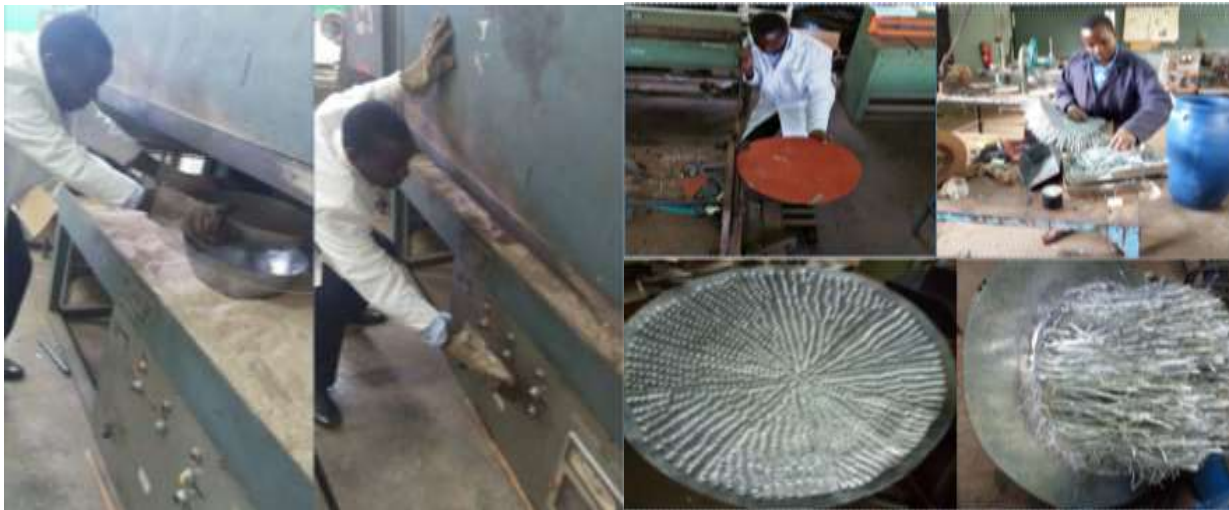
Plate 8-4: Moulding solar collector glazing in annealing oven and Fabrication of collector plate and finned elements surfaces
