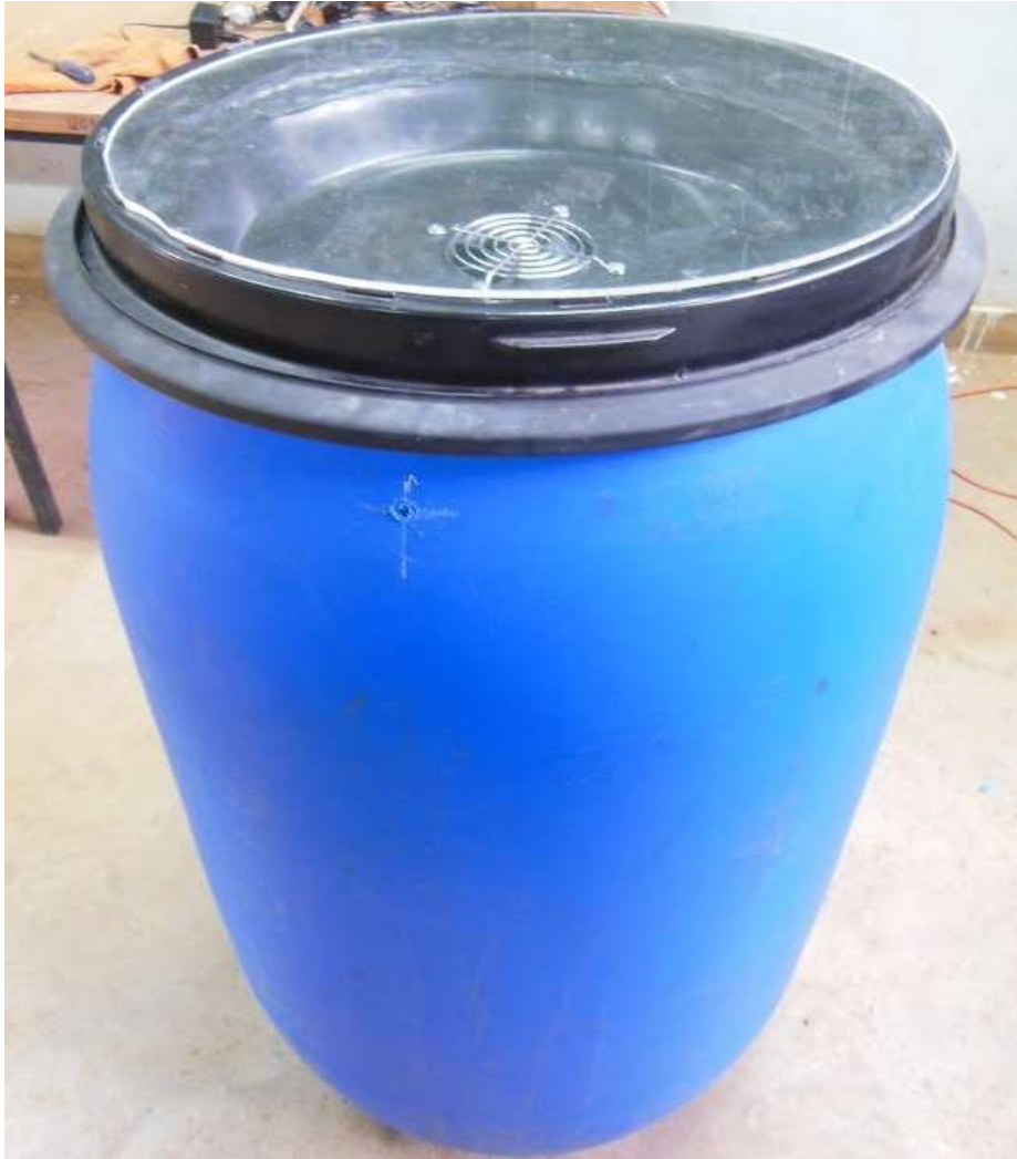
Plate 8-3: Initial existing dryer bin
