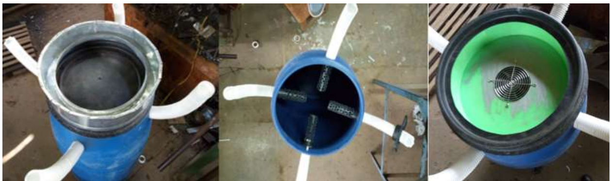
Plate 8-5: Exhaust regeneration conduits fabrication
