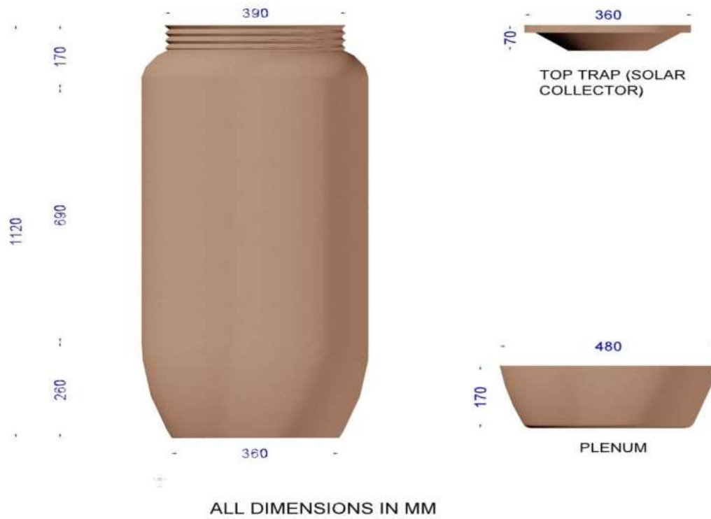
Figure 8-1: Dryer bin compartment dimensions
