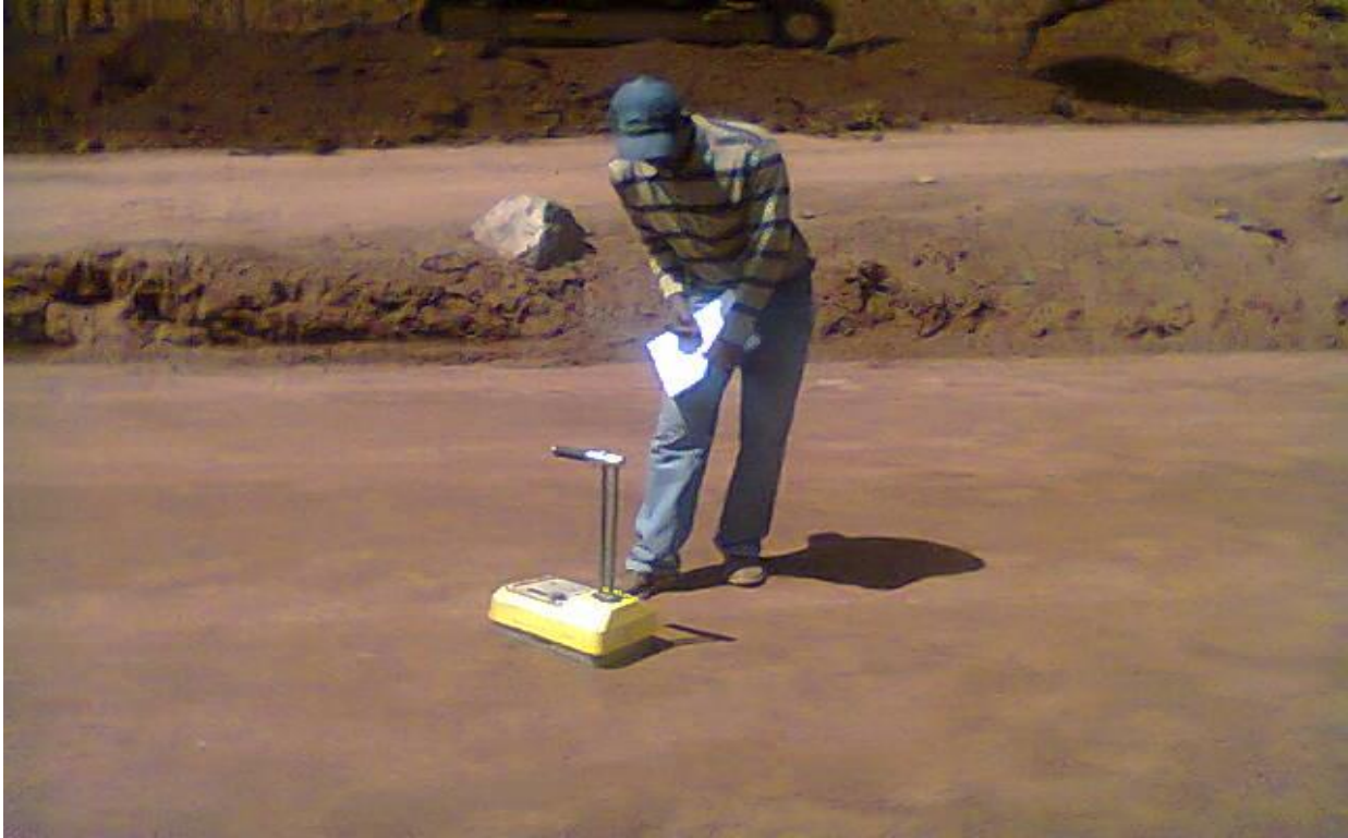
Figure 1-3: Technician recording Readings from a Nuclear Density Gauge.
