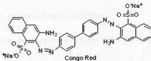
Figure 2: Structure of Congo red dye
