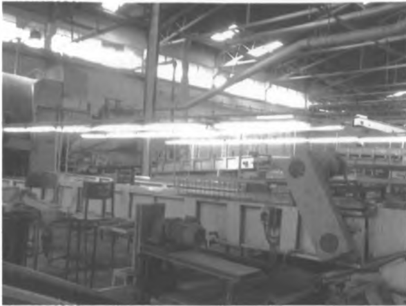
Photograph 4.13 Lights for visual inspection of product
