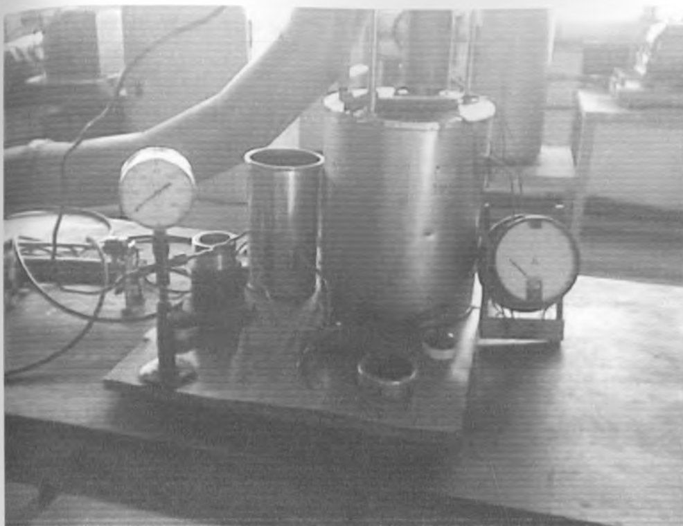
Photo No. 2 Bomb calorimeter used to determine the calorific value
