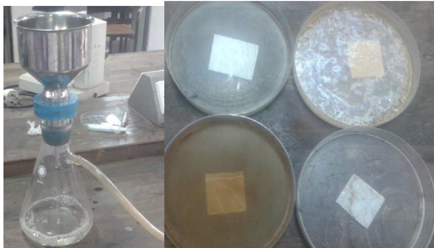
Figure 8: Measurement of Total Dissolved Solutes (TDS) in the laboratory. The filtration apparatus contains water sample after filtration while labeled petri-dishes indicate presence of the sample left after drying in the oven respectively.
