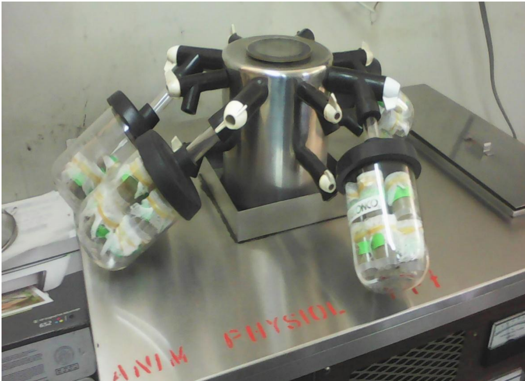
Fig 6: Samples in freeze-drying flasks mounted onto the freeze-drier at RBU. Photo: Peter Oduor.
