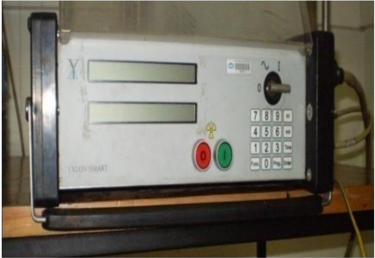
Figure 3.14: Radiography- X-Ray control unit; Model; 583, Manufacturer; Gilardoni, Country, Italy.
