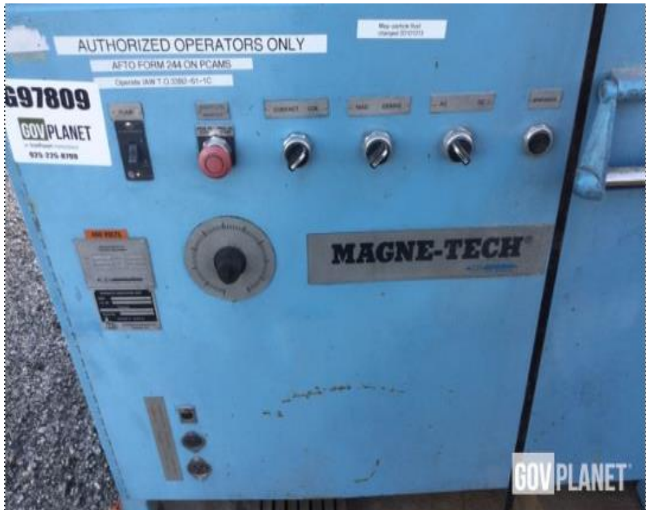
Figure 3.6: The Stationary MPI equipment: Model; GB-3509-01, Manufacturer; Gould Bass Company; Georgia, USA.
