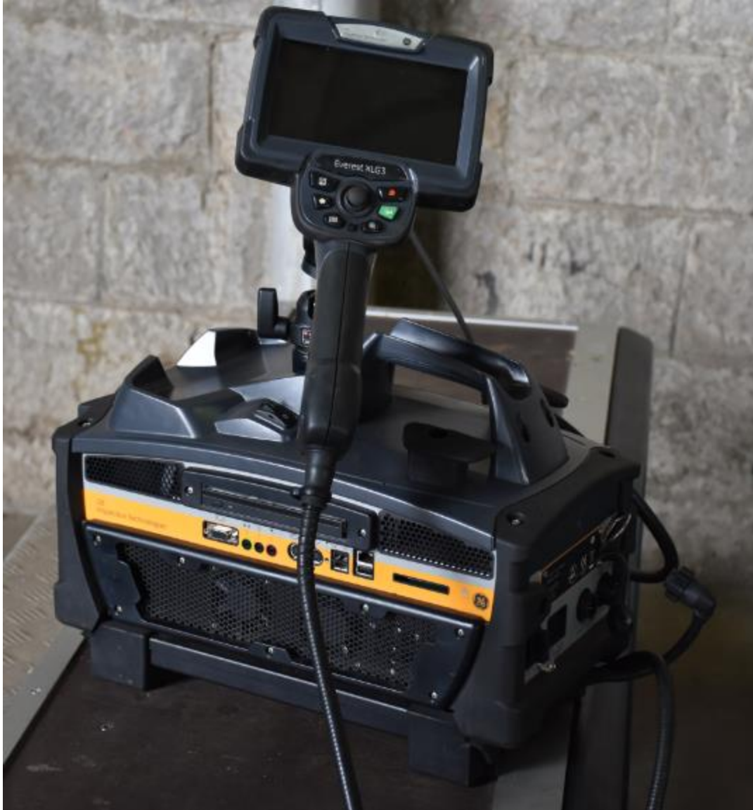
Figure 3.12: Photo of Everest Borescope, Model; XLG3 Videoprobe, Manufacturer; General Electric Company, USA (Extract from Equipment Operating Manual).
