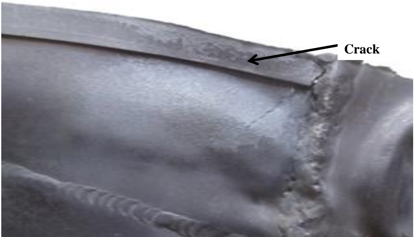
Figure 4.6: Boroscopic Image showing Transverse Crack defect in the Engine Exhaust Section.
