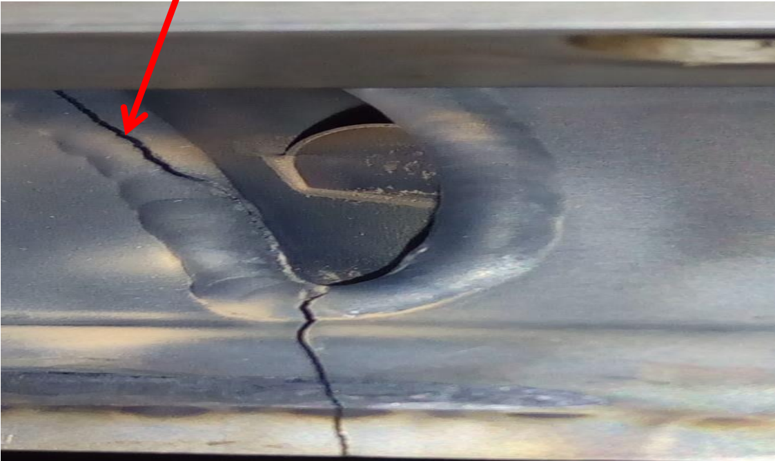
CRACKS AND BURNOUT VIEWED FROM FRONT AND SIDE
