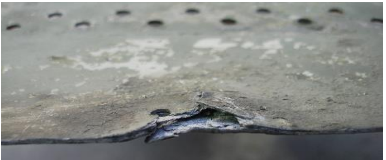
Figure 4.10: A disbond defect in the other Engine Sections.
