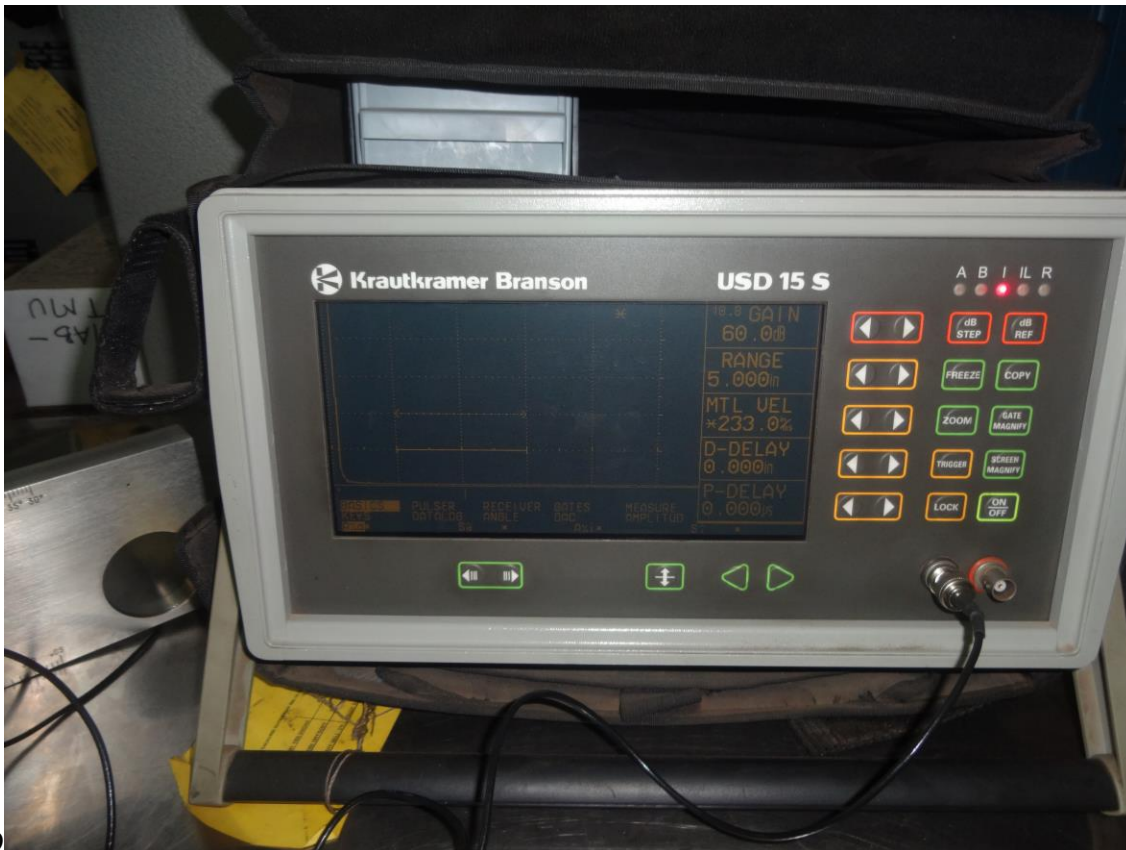
9 Figure 3.9: The ultrasonic inspection equipment: Model-USN 60I 5W ND, Manufacturer; Krautkramer Branson, Australia.
