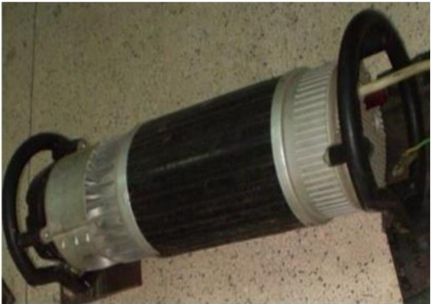
Figure 3.13: Radiography-X-Ray machine (X-Ray Control Unit), Model; Film Type, Manufacturer; Gilardoni, Italy.
