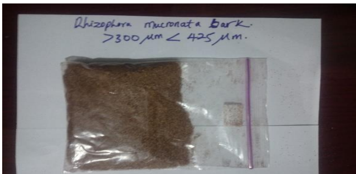
Figure 3.4: Prepared R. mucronata adsorbent stem-bark of particle size, > 300\mu\text{m} < 425\mu\text{m} .
