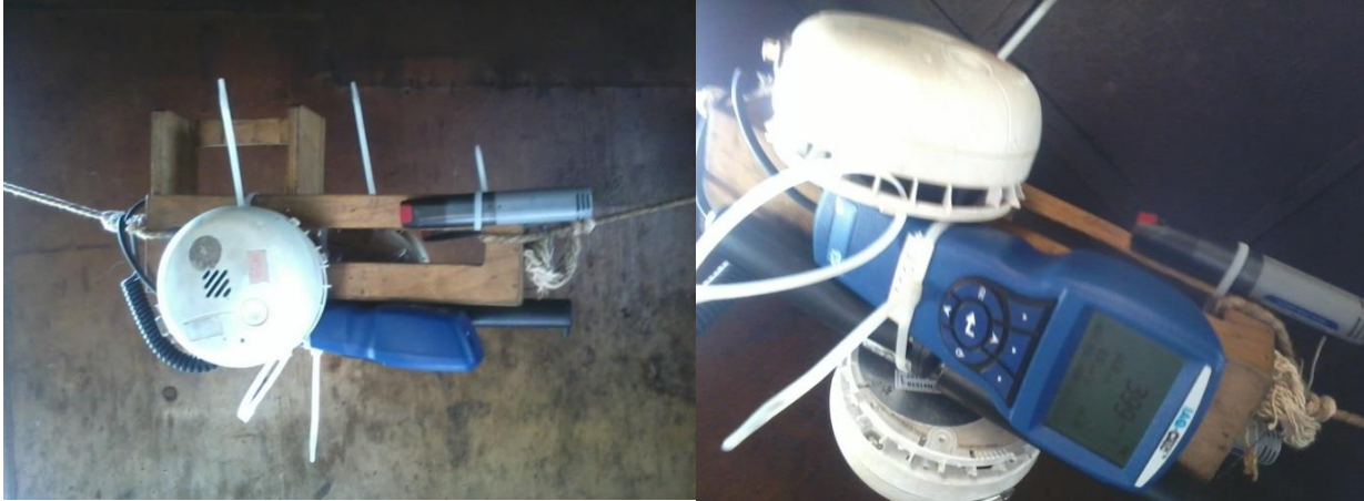
Figure 3-4: Pictures of a CO hobo meter (left) and of a particulate matter meter (right).
