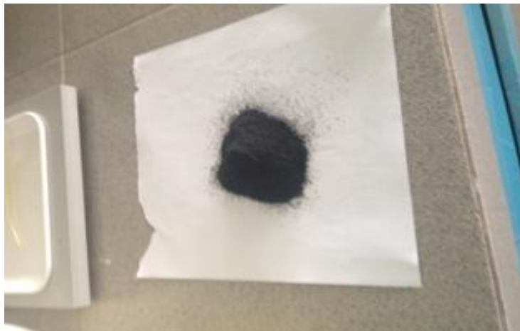
Figure 7: Activated carbon from dry Luffa sponge
