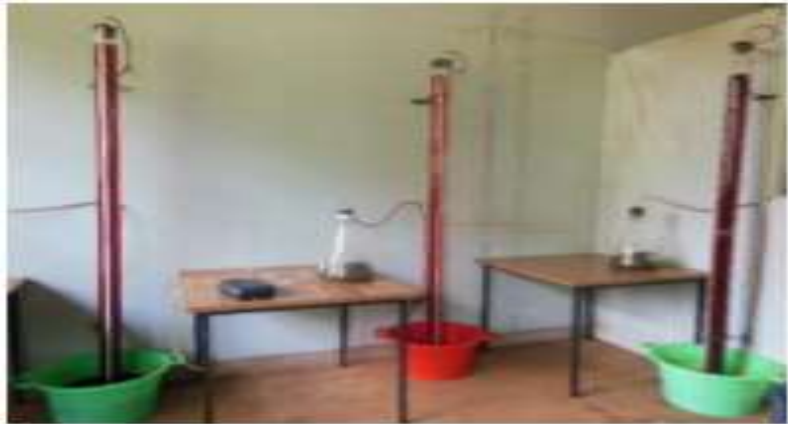
Figure 5: Experimental set-up for low solids anaerobic digestion
