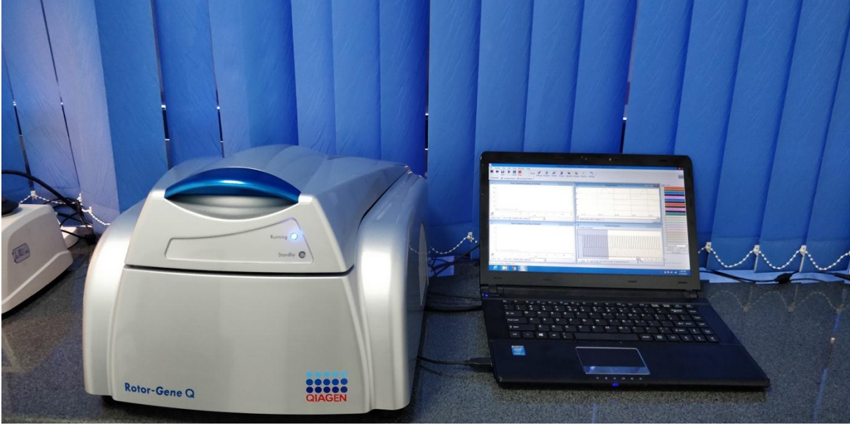
Figure 5: Rotor-Gene Q, QIAGEN Real-time PCR cycler
