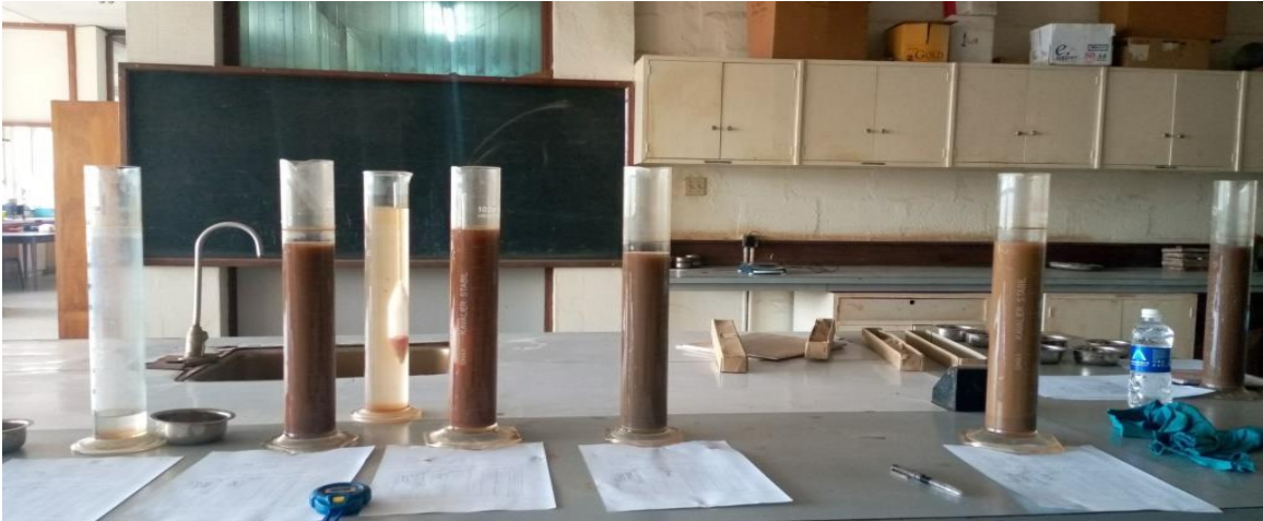
Plate 4.7: Soil solutions ready for hydrometer particle size analysis
