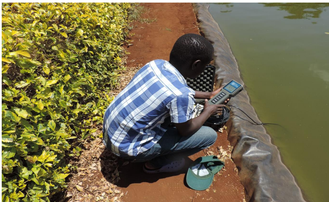
Plate 4: Measurement of physic-chemical parameters using Multi-meter probe at Francis Wahome's pond in Tetu division, Nyeri County (Photo credit: Kashim Oginga)
