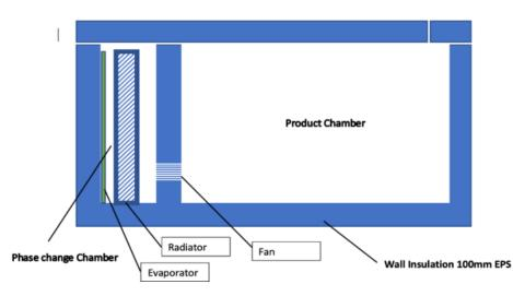
Figure 1. Schematic diagram of the solar cooler.
