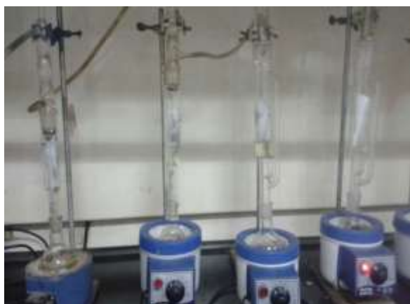
Figure 6. Soxhlet extraction experiment for the residues.
