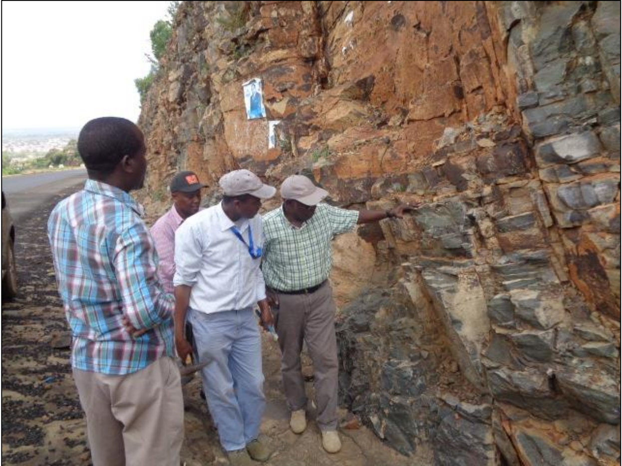
Figure 2.1. Andesitic rock outcrop in Kisumu. The columnar joints and fractures increase the secondary porosity
