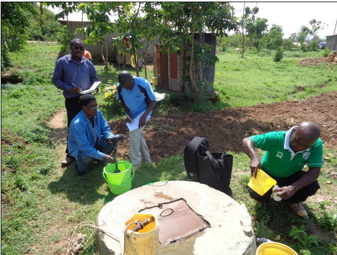
Figure 4.27. Collection of physico-chemical data in Kisumu using Hydrolab Quanta multi-parameter kit.
