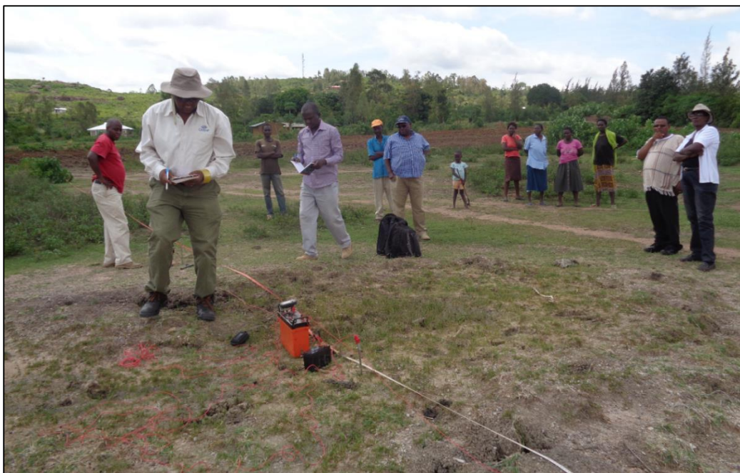
Figure 4.6. VES survey in Kisumu using the Schlumberger configuration, with a maximum AB/2 of 50 meters.
