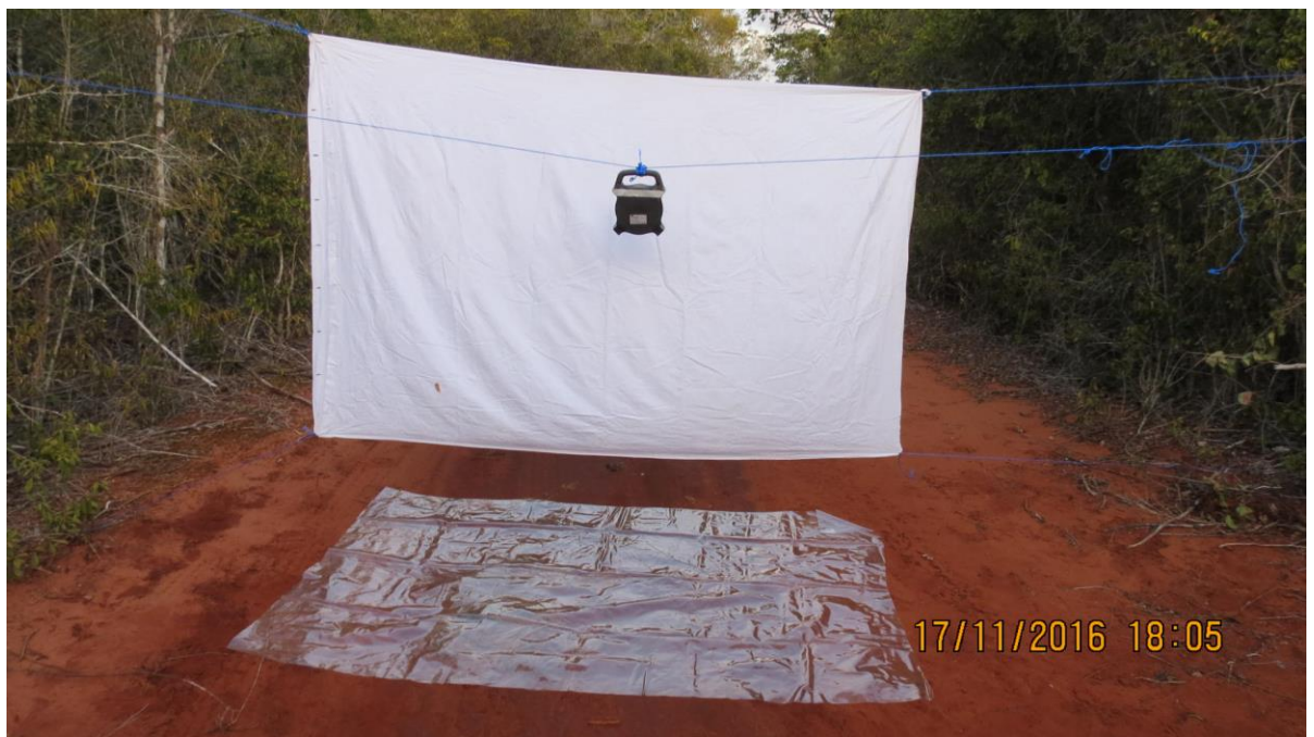
Figure 22. Set up of solar light trap, with white cloth screen and plastic sheet on the ground
