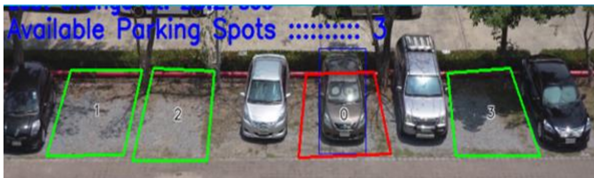
Figure 18: Image of Video Stream Output of detected parking spots, vacant spots and parking count
