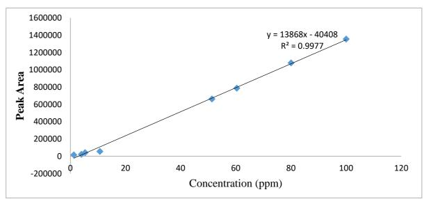
Figure 3b: Calibration Curve for Cypermethrin
