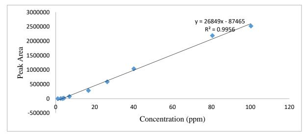
Figure 3c: Calibration Curve for Deltamethrin
