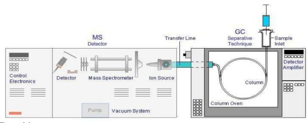
Theory.labster.com Figure 2. 8. Components of GC –MS instrument
