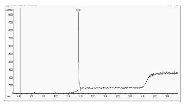
Figure 4 a: The chromatogram for Amitraz Standard
