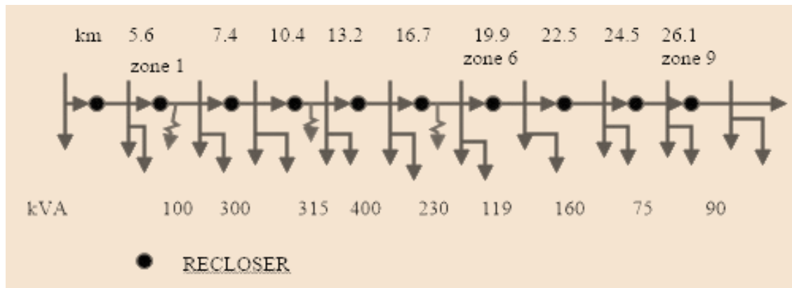
Figure 2.3: Fault Location along the proposed System Network
