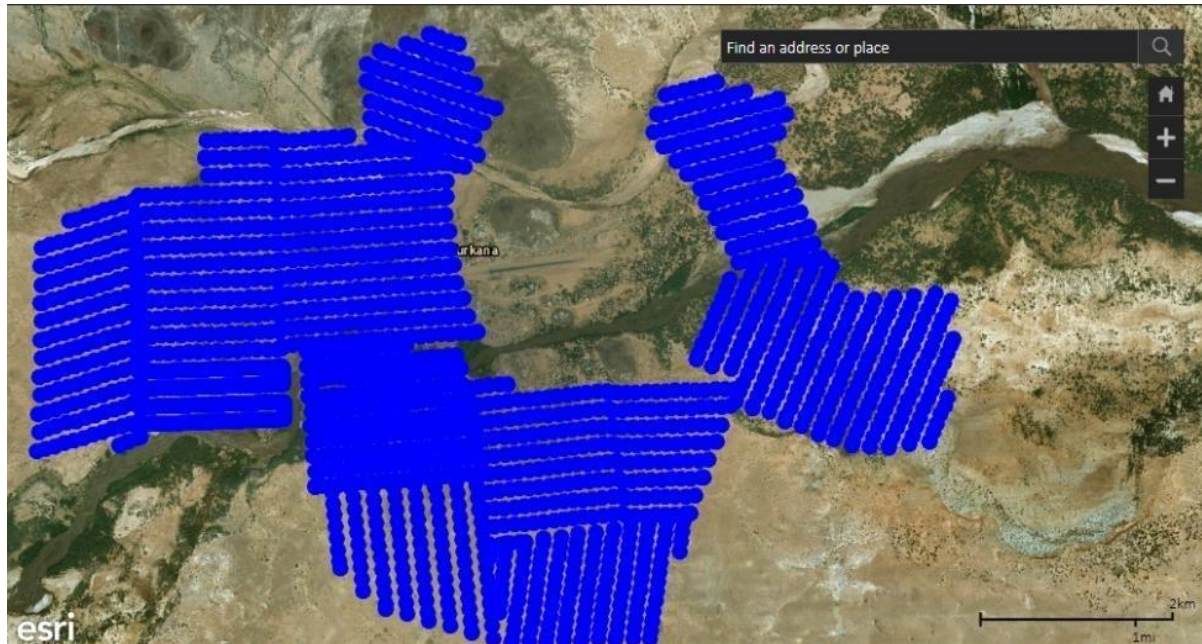
Figure 3.10: Flight paths for the drone during the flight mission in Lodwar town overlaid on the ESRI satellite imagery
