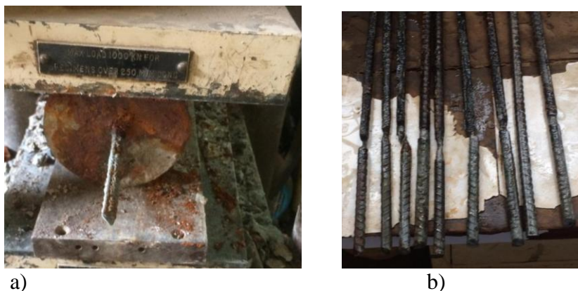
Figure 3.5:(a) recovering the corroded steel, (b) cleaned rebar's for gravimetric weight loss
