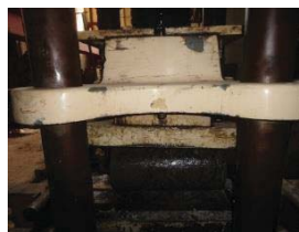
Figure 3.2: Sample during split tensile test
