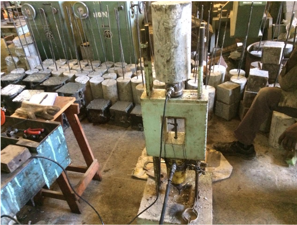
A picture showing a sample during pull out test for bond strength
