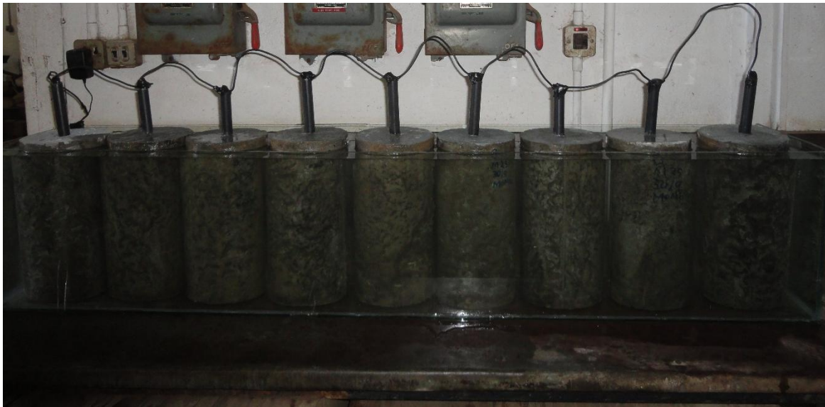
a) A picture showing samples connected in series during accelerated corrosion experiment
