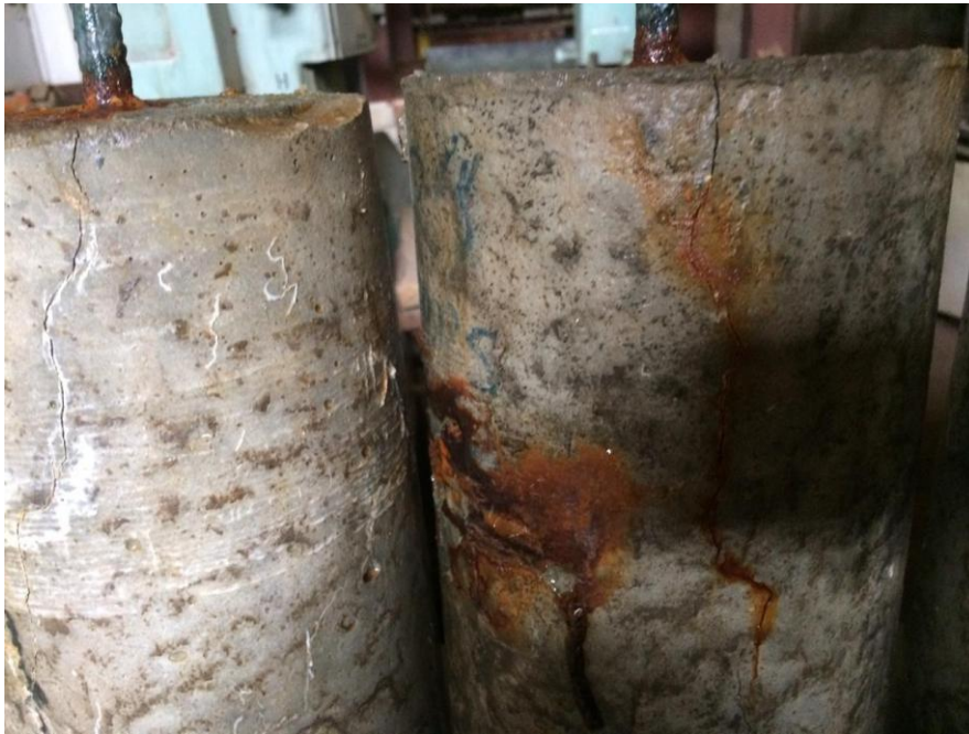
d) A picture showing samples with a longitudinal crack
