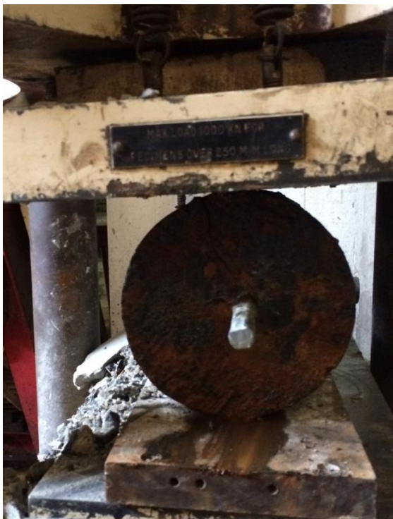
e) A picture showing recovery of embedded steel after accelerated corrosion
