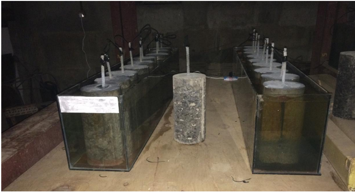
b) A picture showing samples during accelerated corrosion experiment
