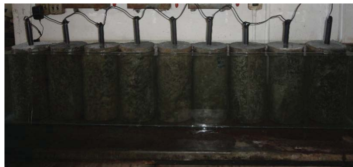
Figure 3.2 Samples of the concrete cylinders in accelerated corrosion set up.
