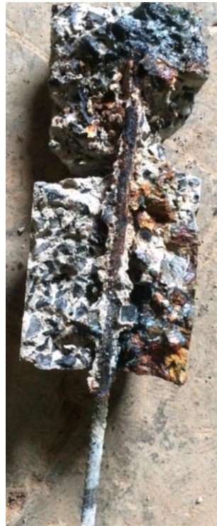
e) A picture showing recovery of embedded steel after accelerated corrosion
