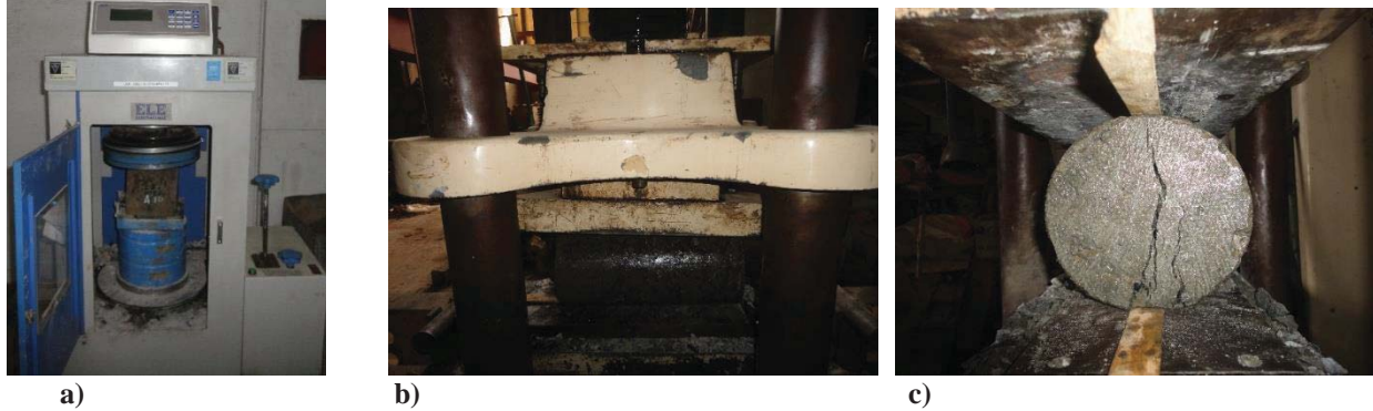
Figure 2:a) Compression testing machine used in the research, b) and c) Failure mode during split tensile test
