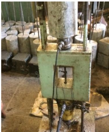
(a) Sample confining apparatus (b) Tensile load detection equipment
