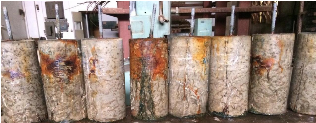
c) A picture showing samples after accelerated corrosion experiment
