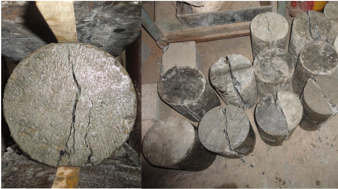
c) A picture showing a mode of failure during split tensile test
