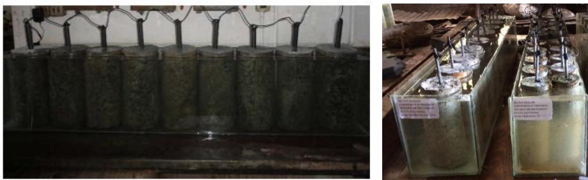
Figure 3.3:(c) Accelerated corrosion set up during experimentation.
