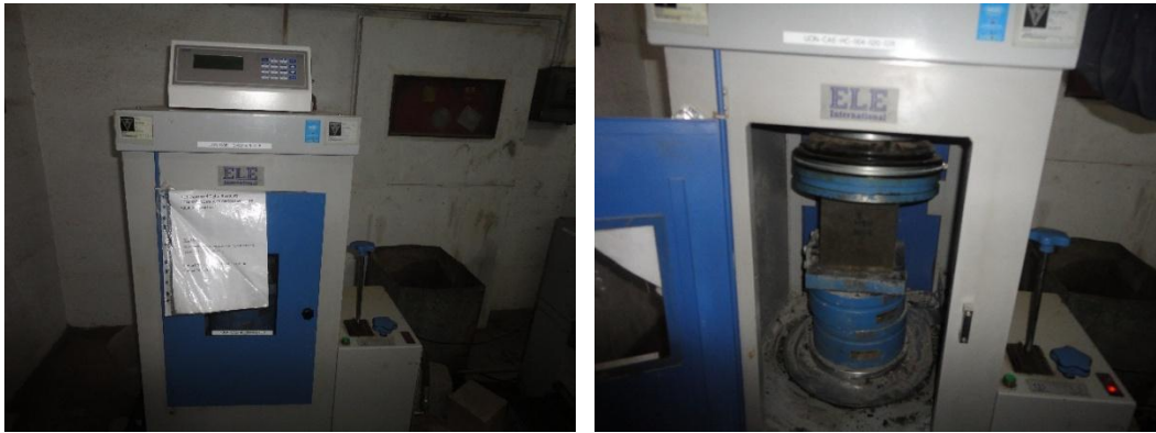
Figure 3.6: Digital compression machine for testing cubes
