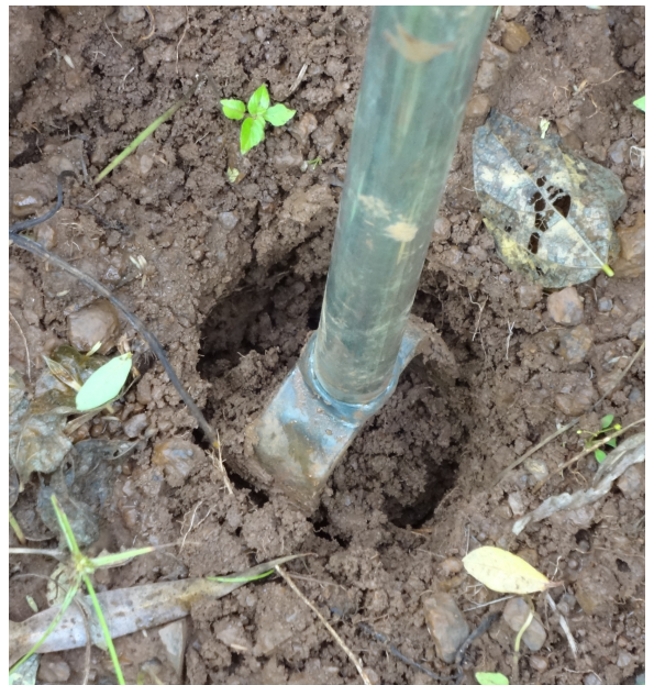
Plate 4.4: Soil auger used to extract samples from the 2.5 m 2 plots for characterize soil properties for the farm survey.
