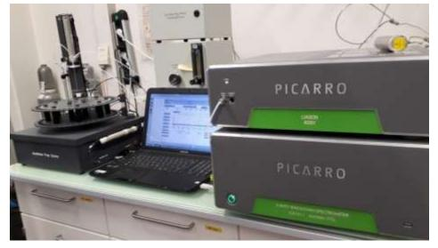
**Figure 3.4:** Picarro cavity ring-down spectrometer (G2101-i Isotopic CO<sub>2</sub>). (*Courtesy of Institute for Geology, University of Hamburg, Germany*)
