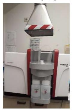
**Figure 3.7: Contra AAS graphite furnace (HR-CS- AAS 800 G; Jena Analytik).** (*Courtesy of Institute for Geology, University of Hamburg, Germany*)
