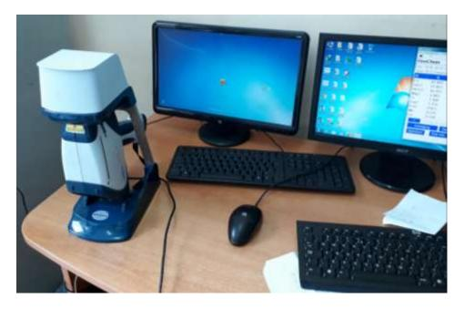
**Figure 3.10: Portable XRF Analyzer (BRUKER S1 TITAN 800).** (*Courtesy of Geochemistry Laboratory at the Ministry of Petroleum and Mining, Kenya*)
