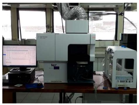
**Figure 3.8: ICP-OES instrument (Agilent Technologies 5110).** (*Courtesy of Kenya Bureau of Standards, KEBS, Kenya*)
