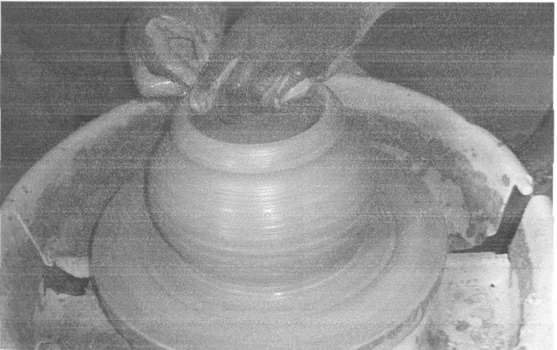
Illustration 33: Throwing done on an electrical wheel
